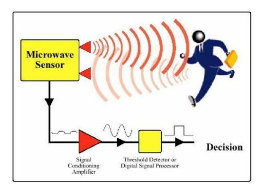
HB100 microwave modules using Doppler radar (Doppler Radar) design principles, mainly used in the automatic gate control switch, security system, the ATM ATM automatic recording control system, automatic train signal etc. places. The HB100 is standard 10.525GHz this detection method has the following advantages compared with other detection methods:
